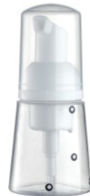
PY012C-35 Capacity:35ml Mouth Dia.:Ø28/410 Bottle Size(AxH): Ø30x60mm Bottle Weight:12g
