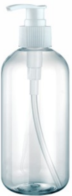
PY002A-400 Capacity:400ml Mouth Dia.:Ø28/410 Bottle Size:Ø66x155mm Bottle Weight:39g
