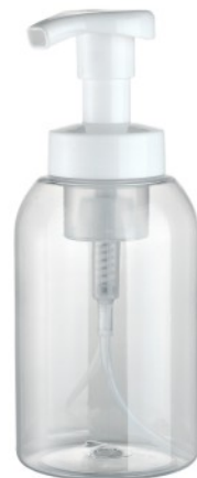
PY012D-300 Capacity:300ml Mouth Dia.:Ø33/410 Bottle Size(AxH): Ø68x121mm Bottle Weight:31g
