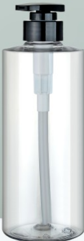
PY004A-600 Capacity:600ml Mouth Dia.:Ø32/410 Bottle Size:Ø73x185mm Bottle Weight:65g
