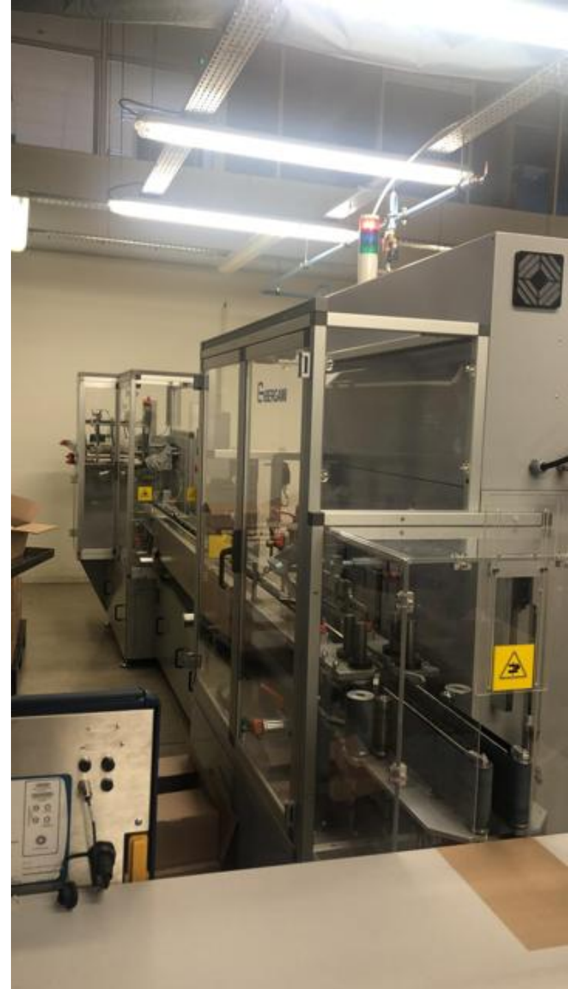
OUTER BOX BUILD UP MACHINE
