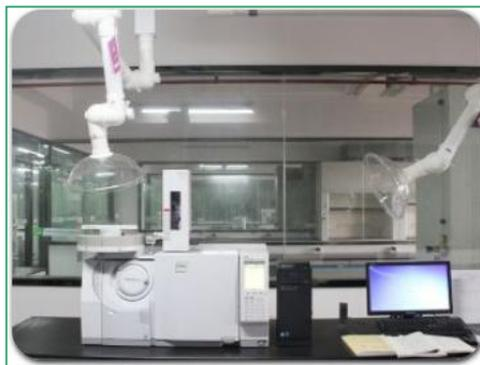
**GCMS QP2010 Plus Gas Chromatograph Mass Spectrometer**
