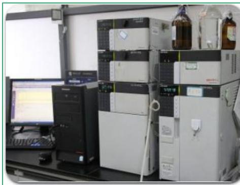
**Shimadzu High Performance Liquid Chromatography**
